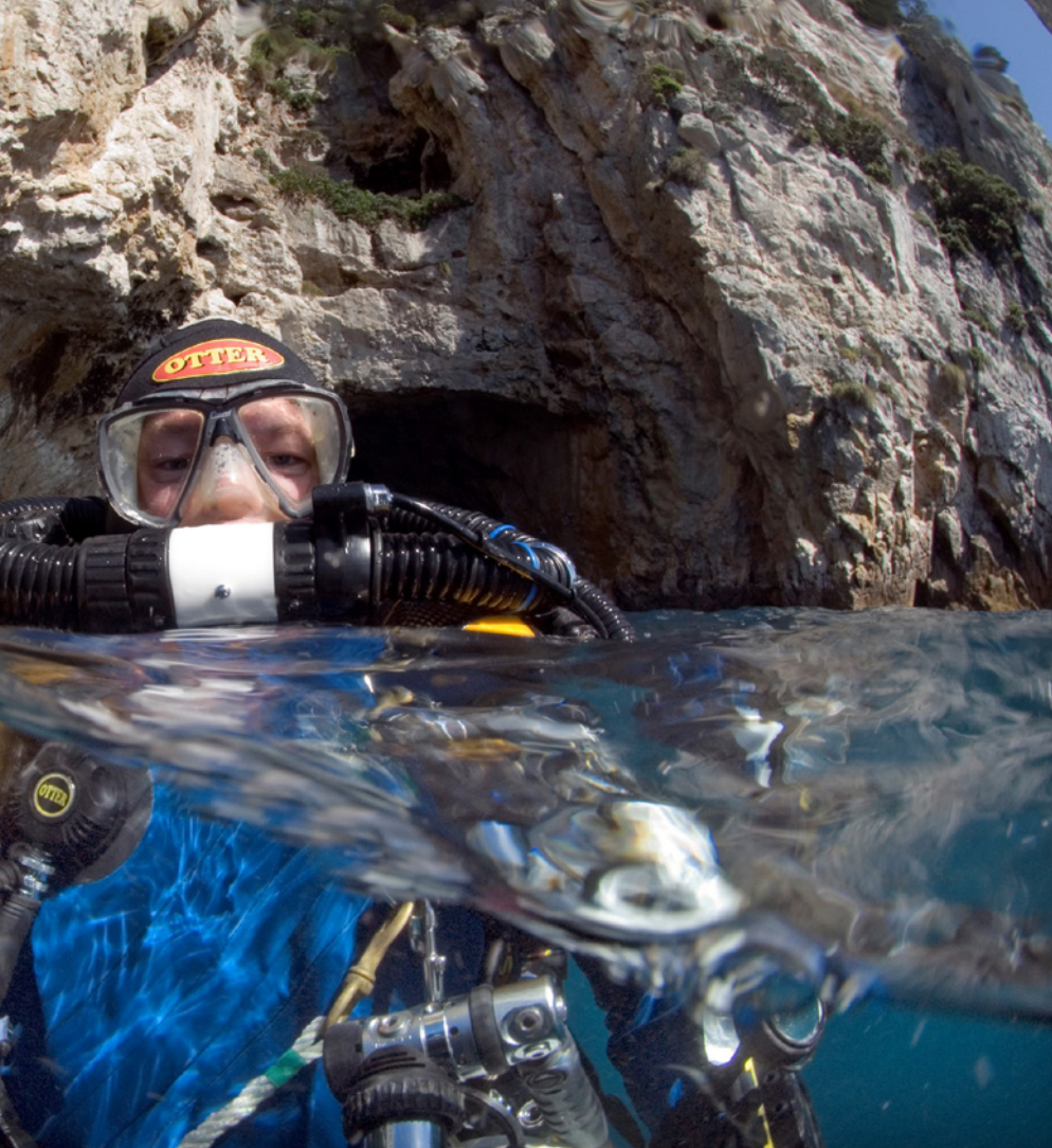
Leigh with his equipment – mixed-gas diving refers to any activity in which the diver breathes a mixture other than air or nitrox – nitrogen/oxygen mixture. The main reason is to avoid nitrogen narcosis. A rebreather absorbs the carbon dioxide in a diver's exhaled breath so the unused oxygen content of each breath can be recycled.
